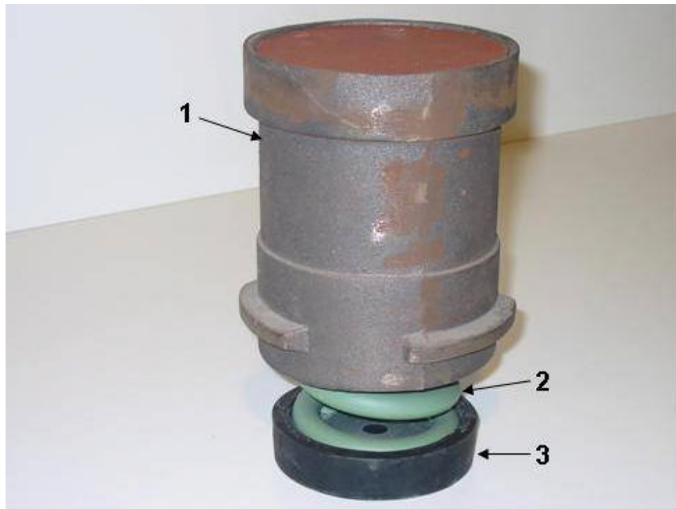
Cylindrical spring housing (screw-type bush, height balance ring, cover) (1), spring (2), support disc with rubber core (3), screwed disc with square hole. The material of the housing is grey cast iron.
